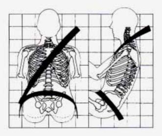
The lap part of the belt should be worn low and snug on the hips, just touching the thighs. In a crash, this applies force to the strong pelvic bones. And you'd be less likely to slide under the lap belt. If you slid under it, the belt would apply force at your abdomen. This could cause serious or even fatal injuries. The shoulder belt should go over the shoulder and across the chest. These parts of the body are best able to take belt restraining forces.
